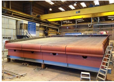
For small to medium power input, the grate has two boiler panels up to 6.4 m wide (left). For larger power input, the grate has four boiler panels up to 12.8 m wide (center and right).
